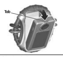
• Pull the tab on the door to remove it.
