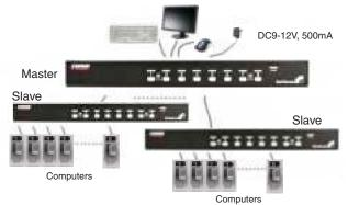
**NOTE:** A device (computer or KVM switch) on any PC port can be changed at any time after initial power up. If you change any one of the PC1 thru PC8 connections from a computer system to a Slave KVM switch or vice-versa, or simply change/replace the device, the On-Screen Display (OSD) will update the next time the OSD menu is activated.
