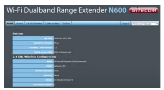
The System status section allows you to monitor the current status of your device, the UP time, hardware information, serial number as well as firmware version information is displayed here.
