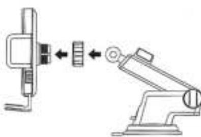
**Step 2:** Fix the base of the suction cup holder at the appropriate position, and press the vacuum switch
