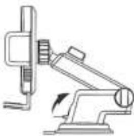
**Step 3:** Turn the knob on the front of support arm clockwise to adjust the height of the support rod
