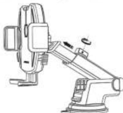
**Step 4:** Turn the knob below the support arm forward to adjust it within 180 degrees.
