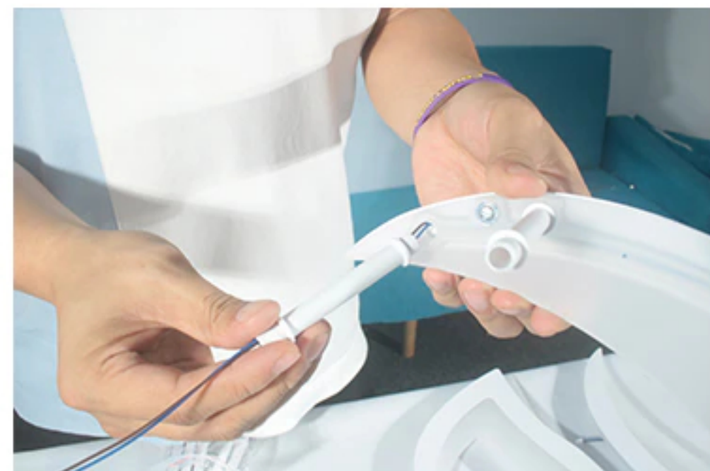
4: Assemble the long tubes to the rest petal, short end of the tubes will be twisted into the petal as well.
