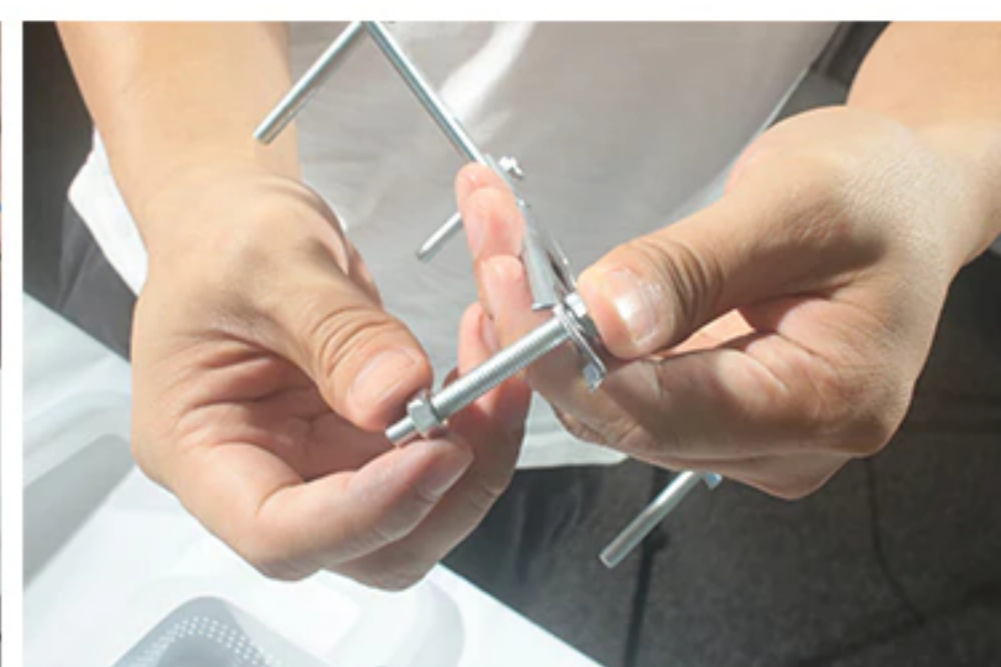
12: Install the screws with flat heads to the cross, use the small nuts to settle the position of each screw.
