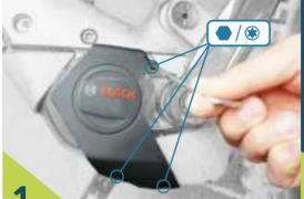
1. Remove cable cover The cable cover of your e-bike can
