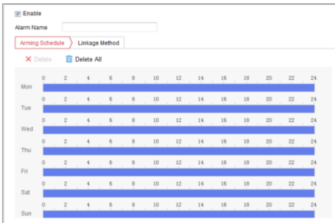
Figure 10-12 Setting PIR Alarm
