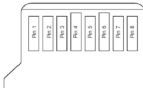
Figure 1: microSD Card Pin Assignment (Back View of Card)
