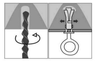
• Drill three holes in the ceiling (make sure there are no electrical wires or pipes in the ceiling), then fix the power line box to the ceiling. Pay attention to the distance between the wall to the heater and the ceiling to the heater:
