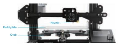
The first and most important step towards ensuring the success of a 3D print is making certain that the build plate is parallel to the plane the extruder nozzle travels in, which is also known as "leveling" in 3D printing. And this is especially crucial and necessary for semi-assembled 3D Printer like Ender-3 without auto-leveling or assisted-leveling feature.
