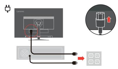
10. Connect the cables with cable clip.
