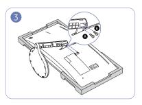
Rotate **A** and **B** screws for fixing.
