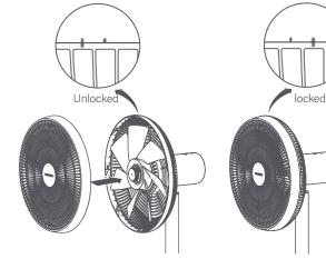
Fix fan grille Insert 8 the screws into the holes on the bottom of the fan cover and screw
