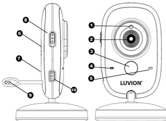
1. **Light sensor** - Allows the baby unit to correct itself under changing light conditions.
