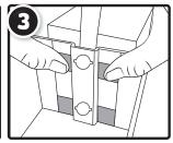
There are four squared marks inside the speaker's walls. When inserting the pegs, press in from both sides.
