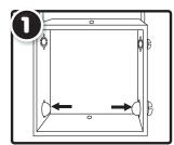
Remove the front cover on the cassette player and push out the bottom pegs.
