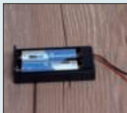
② Put the battery into the battery compartment, pay attention to distinguish between positive and negative
