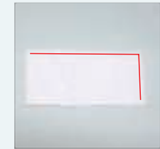
Turn F2 as shown and apply glue according to the red line
