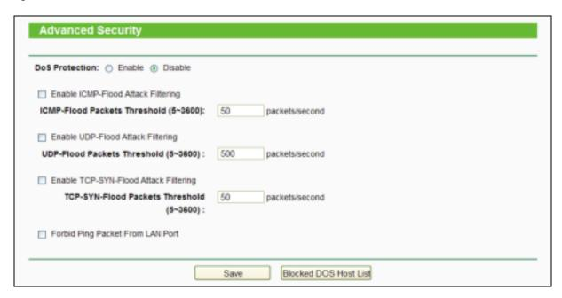
DoS Protection - Denial of Service protection. Check the Enable or Disable button to enable or disable the DoS protection function. Only when it is enabled, will the flood filters be enabled.
