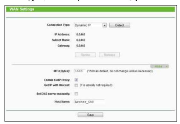
This page displays the WAN IP parameters assigned dynamically by your ISP, including IP address, Subnet Mask, Default Gateway, etc. Click the **Renew** button to renew the IP parameters from your ISP. Click the **Release** button to release the IP parameters.
