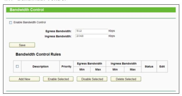
Choose menu "Bandwidth Control", and then you can configure the bandwidth control in the screen as shown in the figure above.
