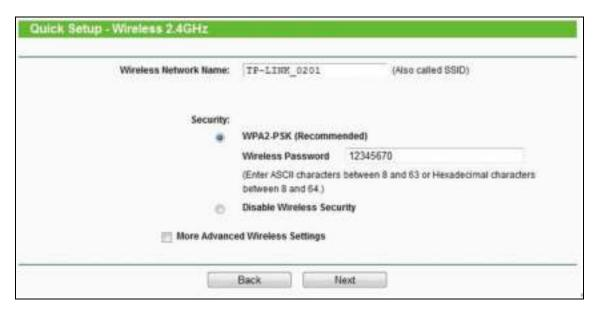
Wireless Network Name - Also called the SSID (Service Set Identification). Enter a value of up to 32 characters. The same name must be assigned to all wireless devices in your network. The default SSID is set to be TP-LINK XXXX. This value is
