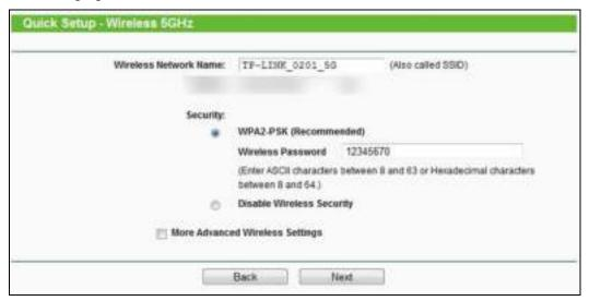
Wireless Network Name - Also called the SSID (Service Set Identification). Enter a value of up to 32 characters. The same name must be assigned to all wireless devices in your network. The default SSID is set to be TP-LINK\_XXXX\_5G. This value is case-sensitive. For example, TEST is NOT the same as test.
