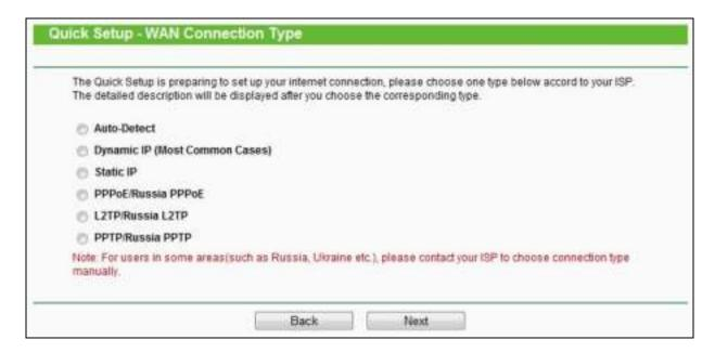
The router provides **Auto-Detect** function and supports five types of WAN connection: **Dynamic IP**, **Static IP**, **PPPoE/Russian PPPoE**, **L2TP/Russian L2TP**, and **PPTP/Russian PPTP**. It's recommended that you make use of the **Auto-Detect** function. If you are sure of what kind of connection type your ISP provides, you can select the very type and click **Next** to go on configuring.
