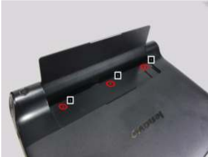
Figure 1-2. Screws on the rear cover
