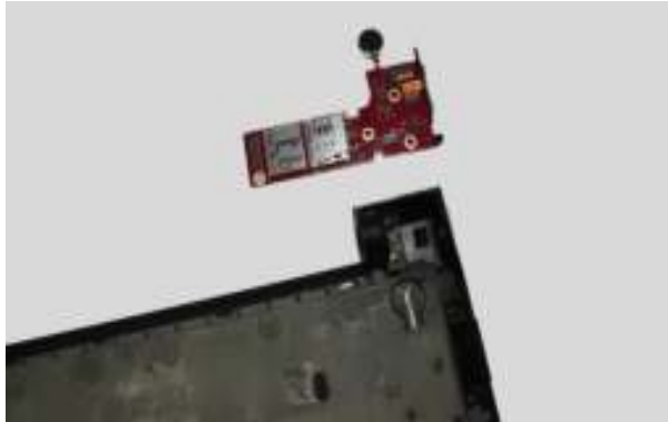
Figure 9-4 Sub board removed
