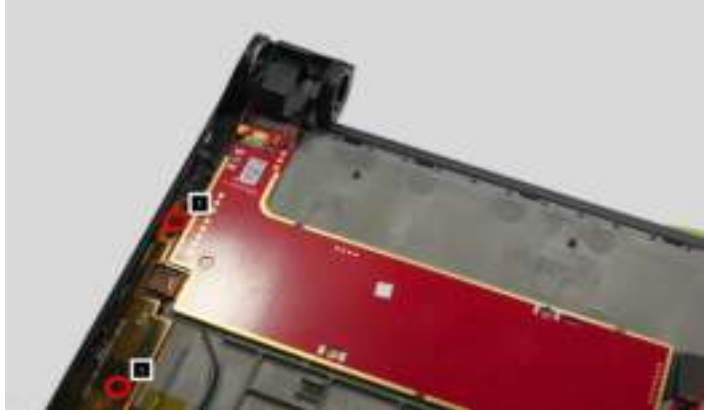
Figure 6-1 Screws on the main antenna
