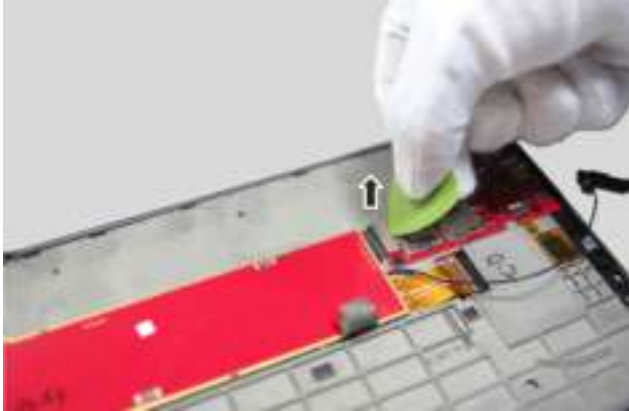
Figure 8-5 Disconnecting the FPC between the main PCBA and sub board
