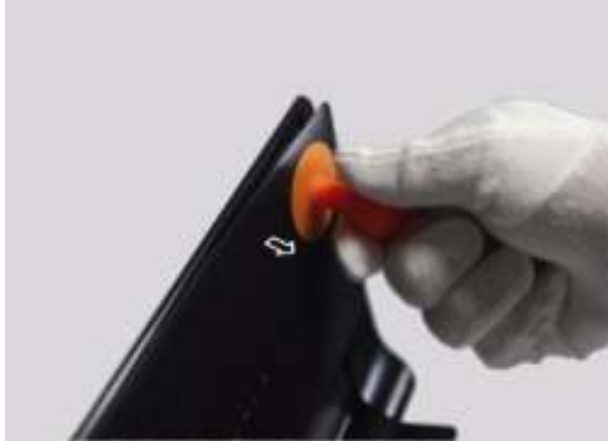
Figure 1-3 Separating the rear cover using a suction tool
