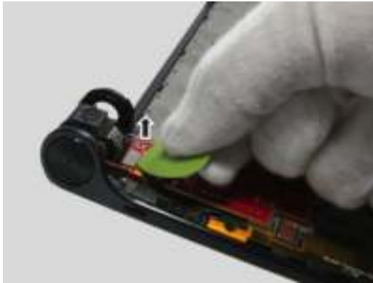
Figure 4-1 Disconnecting the main camera FPC
