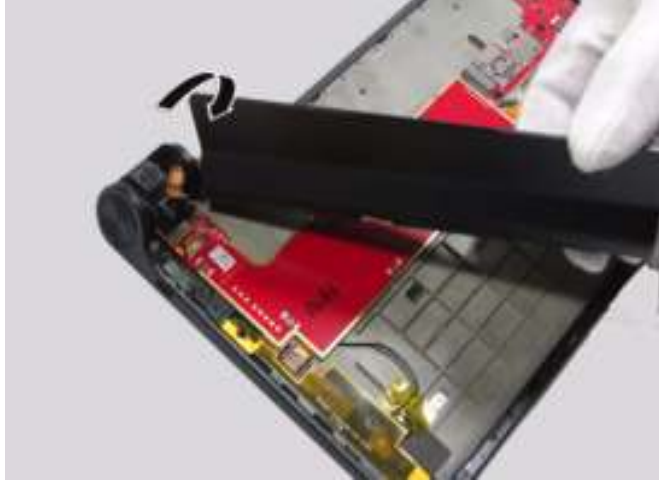
Figure 3-3 Removing the hinge frame with the main FPC at the left end
