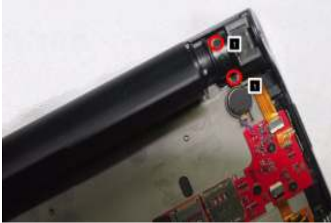
Figure 2-1 Screws on the holder of the speaker box
