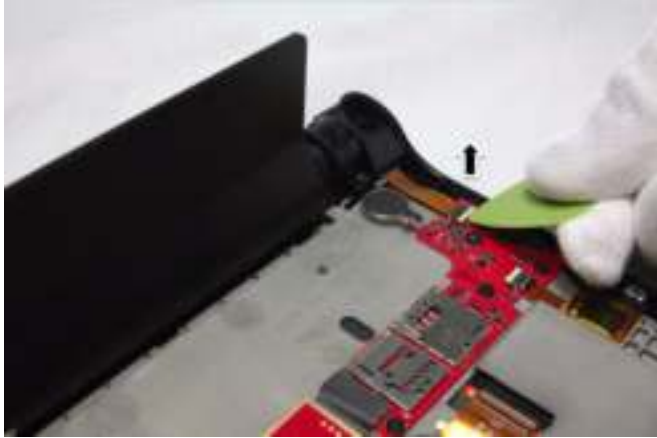
Figure 2-2 Disconnecting the speaker FPC
