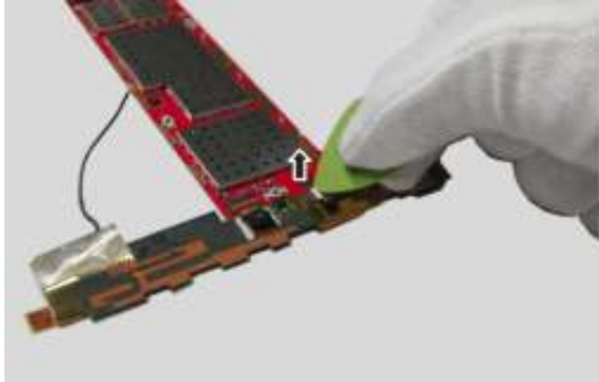
Figure 8-10 Unlock the main antenna FPC connector
