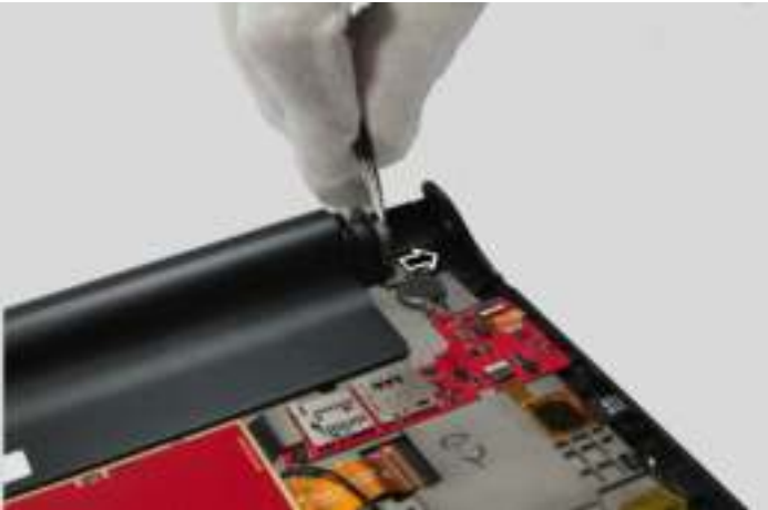
Figure 3-2 Pulling out the hinge pivot
