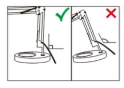
The max angle of the base is  $90^{\circ}$
