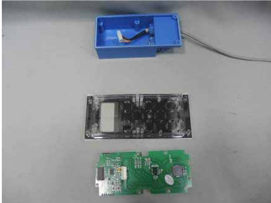
Control box internal view
