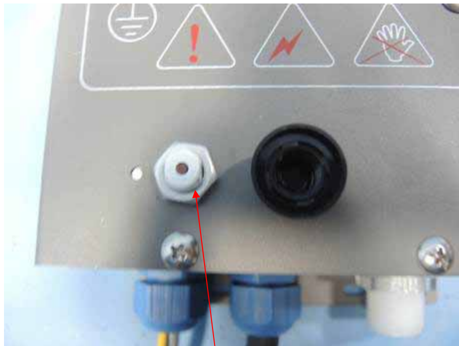
Non Self-resetting thermal cut-out for steam generator (connected to L and N)
