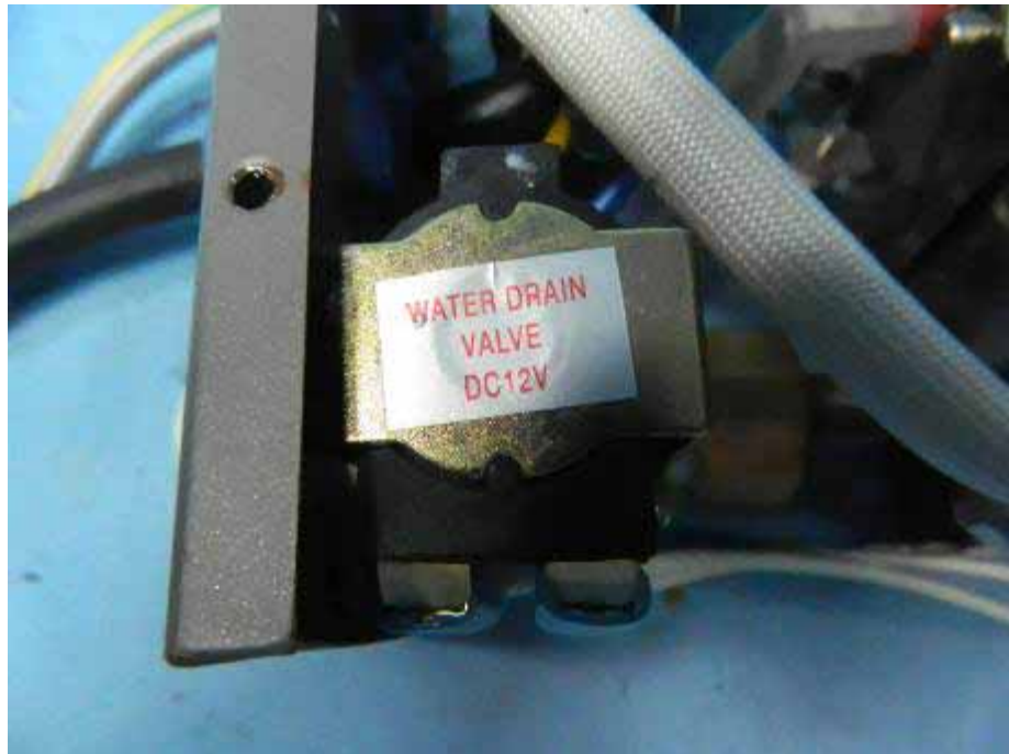
Water outlet valve view
