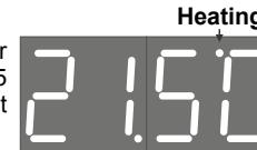
**1 Setting the room temperature.** Click any button. The set value of the temperature 'C' appears and starts to flash. While the value is flashing, through the pressing of the buttons can be changed the set temperature (for auto-repeat the button should be kept). If buttons aren't pressed for more than 5 seconds, then exit from the setting mode is carried out (the value stops to flash).
