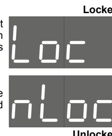
**3 Unlock the buttons.** Turn on the electric heater in the socket during the pressed button '-' and do not release it until corresponding indication and sound confirmation appears.
