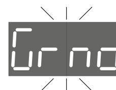
✓ The thermostat, during turning on to the grid and as well during operation can control the presence of ground and during absence, shows the warning (fig. on the left), after which, depending on given function (see below), prohibits heating, waiting for the ground to appear, or after warning permits the work without grounding.
