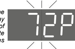
To set the maximum temperature, press any button. It will be displayed and will start to flash the set value of the air temperature in the room 'C'. While the value is flashing at the same time, press and hold both buttons for at least 2 seconds. After the sound signal the set limit value of the surface temperature of the heater 'P' will be displayed and starts to flash. Set the new value and wait 6 seconds to exit the installation mode.
