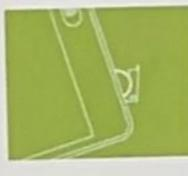
Replace the battery by loosening the screw and pulling it out
