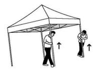
Release auto slider at each corner by pushing Snap-Button to release pressure on slider. Repeat on all four corners.
