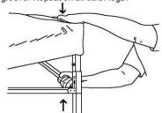
Grasp the bottom of the diamond (shown), on opposite sides. Lift up, and step backwards until shelter is fully opened, being careful not to pinch fingers (for 10'x20' shelter see 2b).
