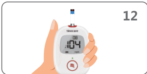
STEP 12: After a 5-second count down, the meter displays the test result.
