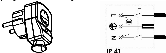
Fig. 1 – VS1 mains plug with the wiring diagram
