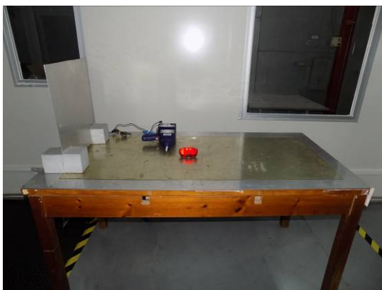
7.3. Photo of electrostatic discharge Immunity measurement (E.S.D.)
