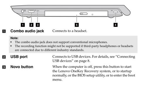
**Kensington lock slot** Attach a security lock (not supplied) here to help protect your computer from theft and unauthorized use.
