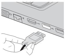
The first time you plug a USB device into a USB port on your computer, Windows automatically installs a driver for that device. After the driver is installed, you can disconnect and reconnect the device without performing any additional steps.
