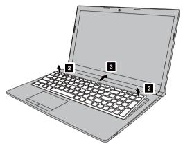
Lift up the keyboard 4 and detach the connector in the direction shown by the arrows 5 6.
