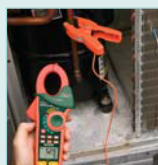
Dual Type K Inputs for taking differential temperature readings needed for superheat measurements.
