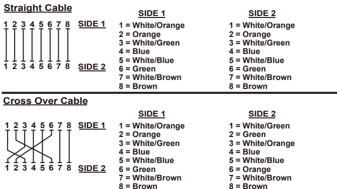
Figure A-1: Straight-Through and Crossover Cable
