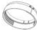
Round fitting for window unit, to be positioned between the end of the tube and the window unit itself
