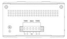
Power can be provided through the dual inputs from separate sources, if needed. One electrical relay can be wired into an alarm circuit. The relay is connected as Normally Closed (will open upon alarm condition).
