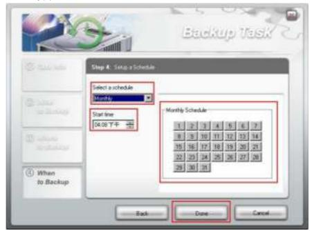
NOTE: The Elite application must be running in order for automatic backup scheduling to work. Scheduled backups cannot be performed unless the StoreJet, JetFlash, and any other hard drives relevant to the files selected in the Backup Task are connected to your computer and powered on.
