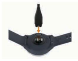
**3** Plug the USB cable into a power source to turn on the device (*Charging the Device*, page 9).
