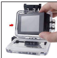
1. Slide the button to the left first. Then, along the direction of the arrow, push up.
