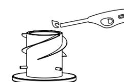
When lighting the combustion gel, make sure to observe sufficient safety clearance. Therefore, only use a long-handled lighter or a long match.
