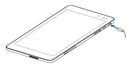
**3** Connect the power adapter to an electrical outlet and charge the tablet until the battery is fully charged.
