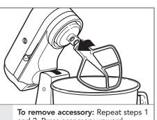
To remove accessory: Repeat ste and 2. Press accessory upward as far as possible and turn to the left. Then pull accessory from the beater shaft.
