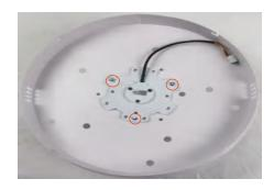
4, assemble the motor to the plate as shown, find the three holes to hold the motor and fasten with the small nuts
