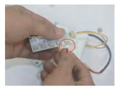
7, connect the all the wires to the collector, pay attention to the direction of each port, Install the plug on the hub to the motor connection
