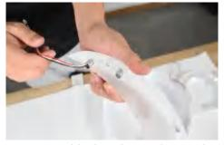
2, assemble the tubes to the petals, each petal has two tubes, the wire of the petal goes through one of the tube
