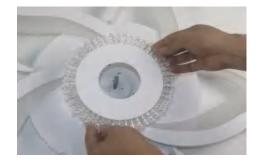
6, assemble the bottom plate to the light, find twist three bolts from the other side to secure the plate
