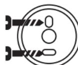
**3.** Carefully tap the plugs into the holes with a suitable hammer
