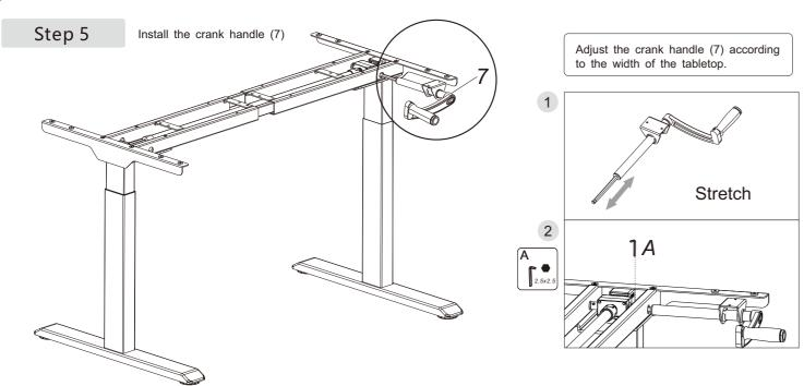
Option 1: Installed the handle on the right side of the table.
