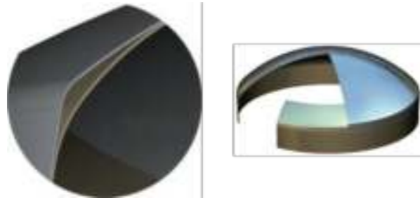
Figure 33 3D CAD sectional views of the tweeter dome and extended former that meet to form a triangular stiffening member at the dome edge
