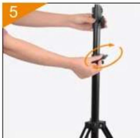
5. Loosen the screw knob on the middle pole to extend the light stand to the height you want
