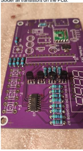
Be careful while soldering the transistors on the PCB, they need to bee cooled a bit during the soldering process!
