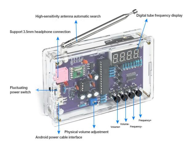
Dual power supply: 5V mobile phone charger or two No. 5 dry batteries
