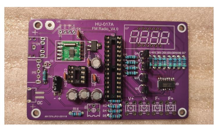
After the ELco's Solder also the IC base sockets for item U2 and U9.
