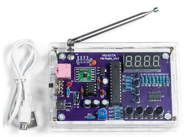
Whit this FM Radio, when it is finished, you can listen to several radio stations transmitted by air in the frequency range of 87-108MHz. So all you favorite stations on this small device! It is a: do it yourself building kit, with all components inside the package! The only thing You need to provide, is a soldering tool with solder, solder skills, a power source and or batteries. Some screwdrivers, cutters etc..
