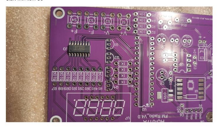
Be sure that the IC 74HC595D is positioned like the picture. Once you have soldered this one wrong it is a disaster to remove and resolder!!
