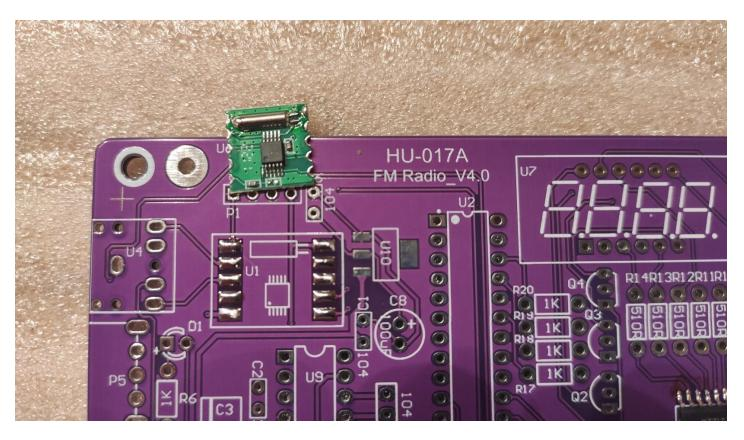
Solder this Radio module on the pcb.
