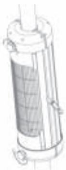
Adjust the position of the radiant heater (at least 50 mm from the floor) and then fix it by turning the two star-shaped locking knobs clockwise.
