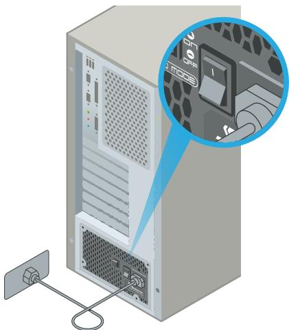
**4.5.** Connect the AC power cord to the PSU. Plug the AC power cord into the wall socket.
