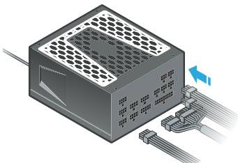
**4.4.** Connect all the necessary system DC cables (Motherboard, CPU, VGA, HDD, Optical Drivers, etc). The connectors should click to lock in.
