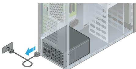
**1.1.** Disconnect your AC power cord from the wall socket and the back of the power supply.
