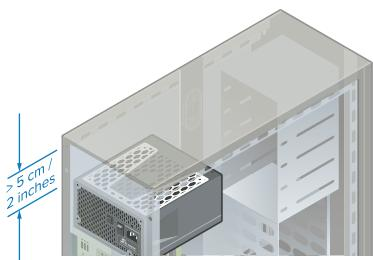
Mount the power supply with the ventilation top cover facing UPWARD only if there is enough space (at least 5 cm / 2 inches) available between the PSU ventilation top cover and the metal plate of the case, and only if the case has a ventilation panel on top.
