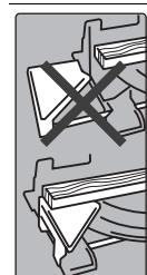
The free end of workpieces must be underlaid or supported by the saw-table extensions.
