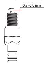
Standard Spark Plug: E6TC/E6RTC/BPR7HS
