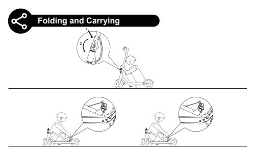
Make sure that the scooter's turned off. To fold, unlock the folding mechanism, and bend the handlebar stem to hook the buckle on the rear fender. To open, press the bell trigger to remove from the buckle, erect the handlebar and lock the folding structure.
