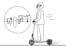
4. Release the accelerator and the kinetic energy recovery system (KERS) initiates automatically to brake slowly; And squeeze the brake lever for a sudden brake
