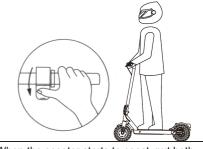
3. When the scooter starts to coast, put both feet on the deck and press the accelerator (the accelerator initiates once the coasting speed exceeds 3mph)
