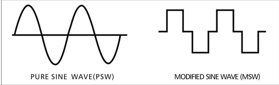
**Modified Sine Wave:** If your equipment can accept some voltage fluctuations, consider a modified sine wave inverter. These inverters provide mobile power at a more affordable price and come in a full range of sizes, from handheld to high performance. Do not use to power sensitive devices such as medical equipment or computers. Some audio equipment may perform poorly if run on Modified Sine Wave power.
